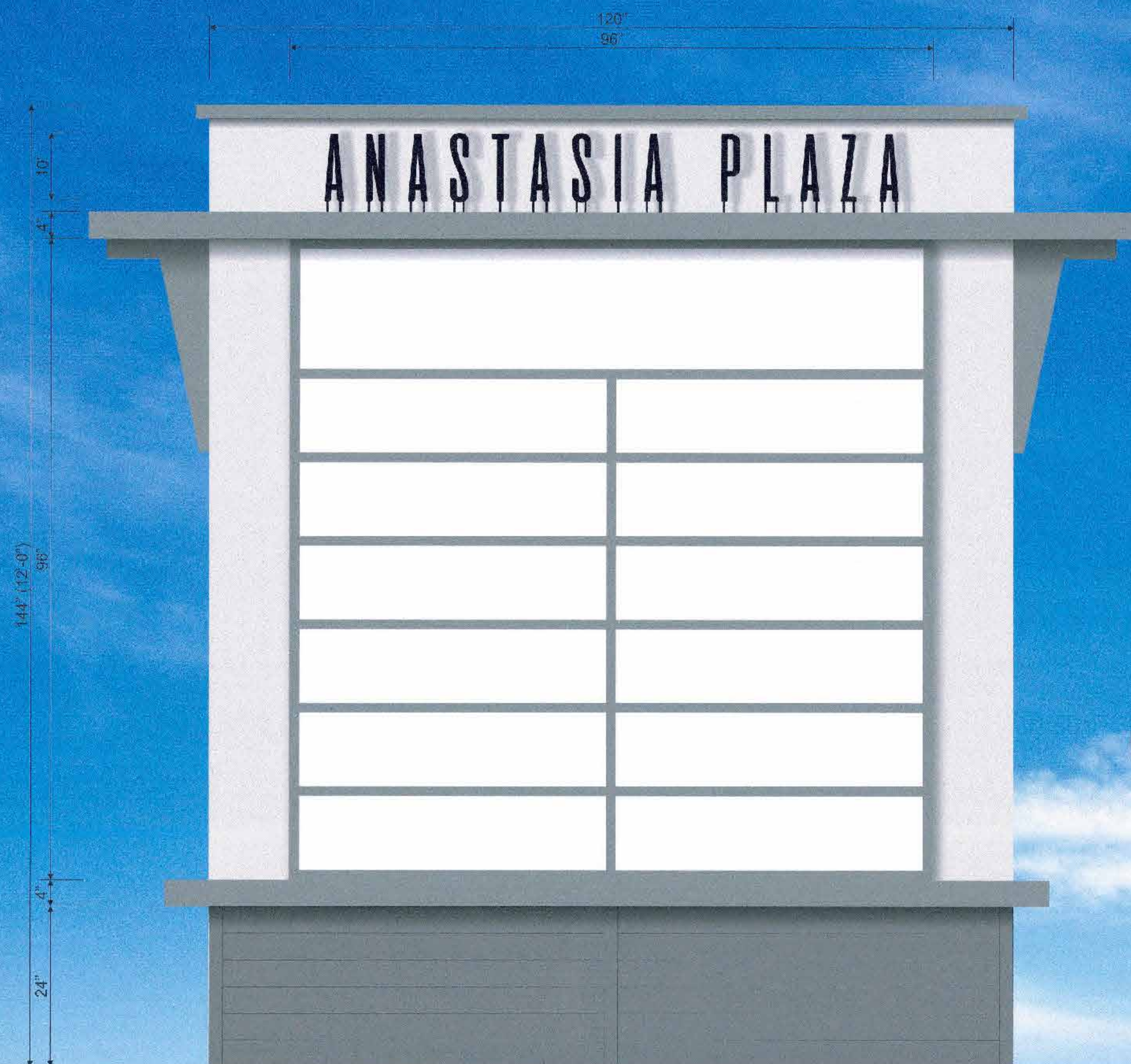
Front Elevation - Illuminated Pylon Sign 1/2" = 1'-0"
