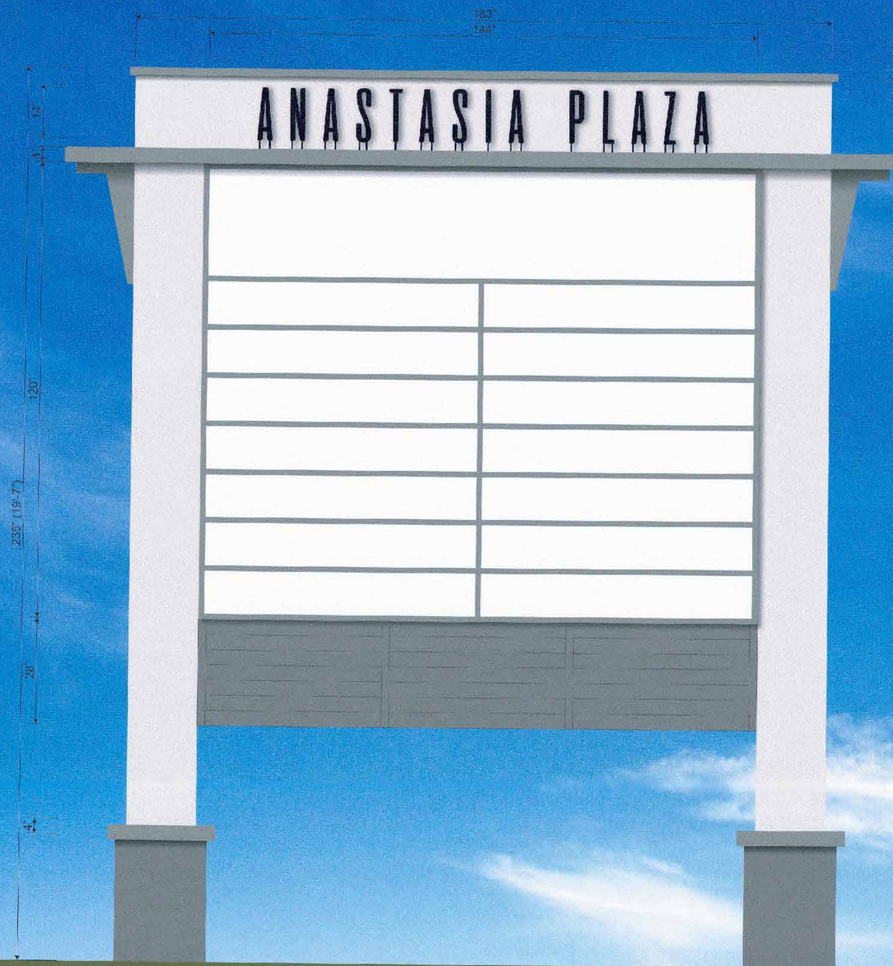
Front Elevation - Illuminated Pylon Sign | 3/8" = 1'-0"
